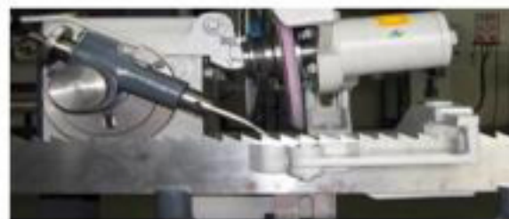
Fast grinding of band saws up to 100mm width.
